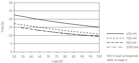
100 % load corresponds to the max. output power (full load) according to the table on page 2.
