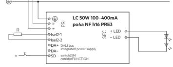
The voltage line for switchDIM / corridorFUNCTION must be the same line as on the mains input of the Driver. In switchDIM applications the DALI interface as well as the integrated DALI bus power supply (IPS) can not be used
