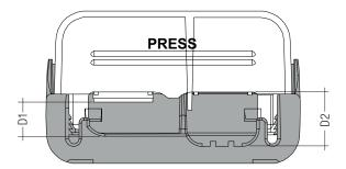
Depending on the used flaps of the terminal following cable jacket diameter difference between the side D2 and D1 terminals is recommended:
