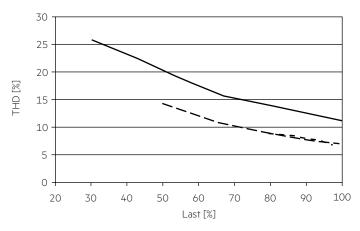
100 % load corresponds to the max. output power (full load) according to the table on page 2.
