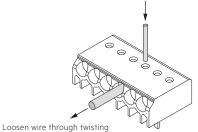
and pulling or using a Ø 1mm release tool
